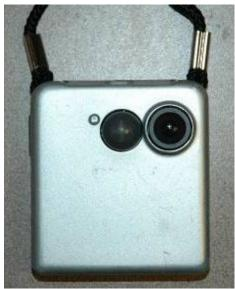
Figure 1. SenseCam (64x71mm body)
